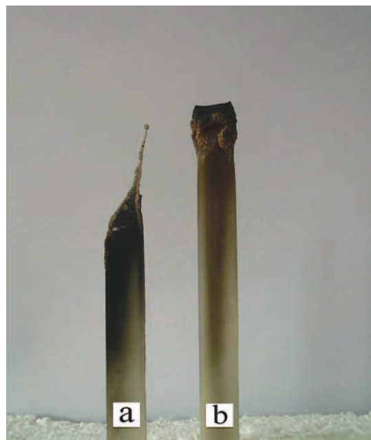
Figure 3 Photograph of the FR-PA6 bars from UL-94 tests. (a) PA6/MgHP; (b) PA6/AlHP. [Color figure can be viewed in the online issue, which is available at wileyonlinelibrary.com.]
